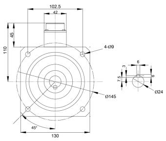
31M-DHT-15 [Rated output: 1.5kW]
